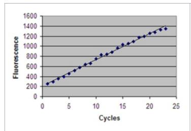
Example of assay result. DUB assay: 50 nM USP2 catalytic domain (BML-UW9850); 500nM Ubiquitin-AMC; 50mM HEPES, pH 7.8, 0.5mM EDTA, 1mM DTT
