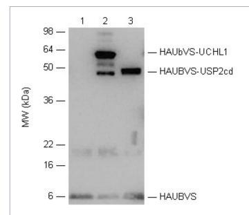
Image: DUB active site probe assay: Western blot showing reactions containing HAUbVS only (lane 1), HAUbVS + GST-UCHL1 (lane 2, Prod. No. BML-UW9305), and HA-UbVS + USP2cd (lane 3, Prod. No. BML-UW9850). HAUbVS modified proteins detected using HA polyclonal antibody (Sigma – H6908) at 1:1000 dilution.""""
