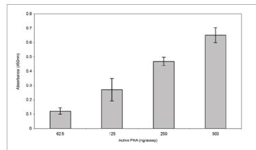
Analysis of purified active PKA activity with EKS-390A. Varying quantities of purified active PKA were assayed using the PKA substrate microtiter plate. Assays were incubated for 60 min. at 30°C.
