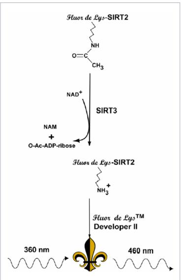
Figure 1: Reaction Scheme of the SIRT3 Fluorescent Activity Assay. NAD+-dependent deacetylation of the substrate by recombinant human SIRT3 sensitizes it to Developer II, which then generates a fluorophore (symbol). The fluorophore is excited with 360 nm light and the emitted light (460 nm) is detected on a fluorometric plate reader. NAD+ is consumed in the reaction to produce nicotinamide (NAM) and O-acetyl-ADP-ribose.
