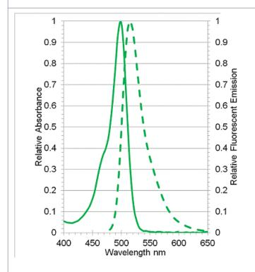
Excitation (solid line) and emission (dotted line) spectra of FLUOFORTE® dye.
