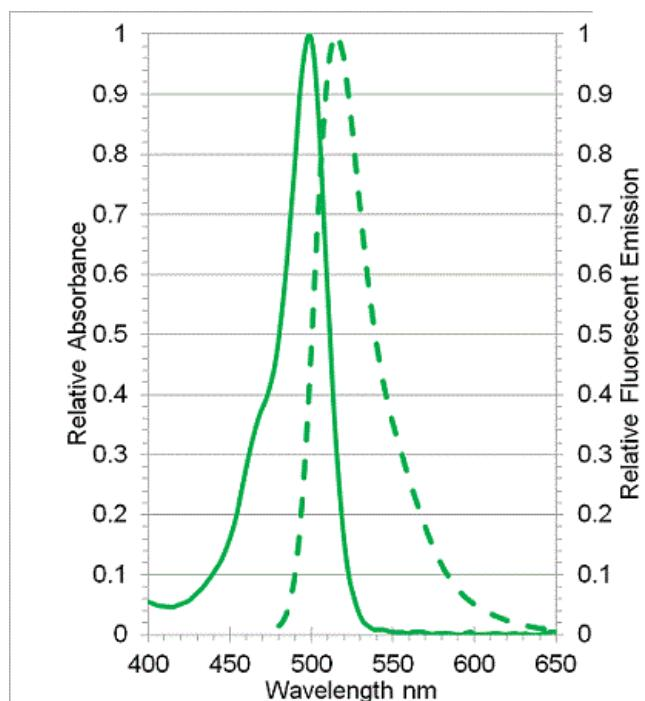
Excitation (solid line) and emission (dotted line) spectra of FLUOFORTE® dye
