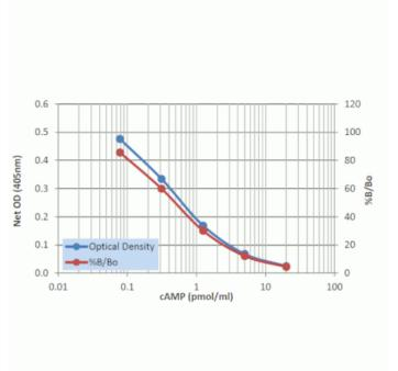
Typical standard curve used to calculate cAMP concentrations for Non-acetylated assay format.
