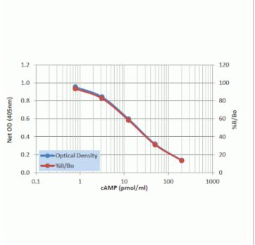
Typical standard curve used to calculate cAMP concentrations for Acetylated assay format.
