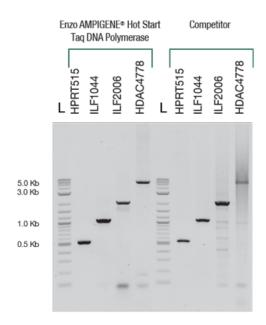
Performance of AMPIGENE® Hot Start Taq DNA Polymerase vs. Competitor. AMPIGENE® Hot Start Taq DNA Polymerase shows strong signal and clear results. Human Genomic DNA (5ng) template was targeted with four separate primer sets in 20µl PCR volume. Annealing temperature was 60°C. 1 kb ladder (L).
