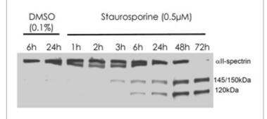
Rat primary septo-hippocampal co-cultures (astrocytes and neurons cultured from day E18 rat embyros) were challenged with the pro-apoptotic compound staurosporine or with vehicle (DMSO) for times indicated above. Protein (40 µg) was separated by SDS-PAGE, transferred to PVDF membrane and probed with FG6090. The caspase-3 cleaved 120-kDa fragment of alpha-II-spectrin was detected at a dilution of 1:4000. Western blot provided by courtesy of Dr Brian Pike, University of Florida.
